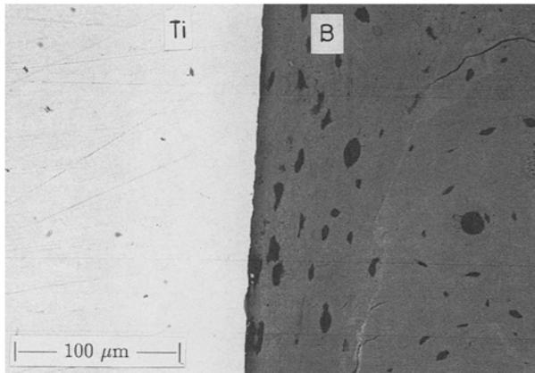
Figure 6 SEM micrograph of titanium cone showing contact, but no bonding, after 8 weeks in rabbit tibia. Ti = titanium, B = bone.
