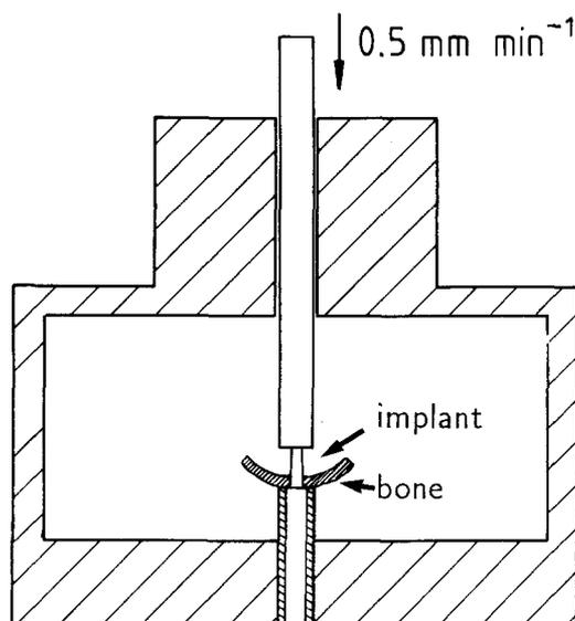
Figure 1 Schematic illustration of a specimen in the push-out test fixture.
