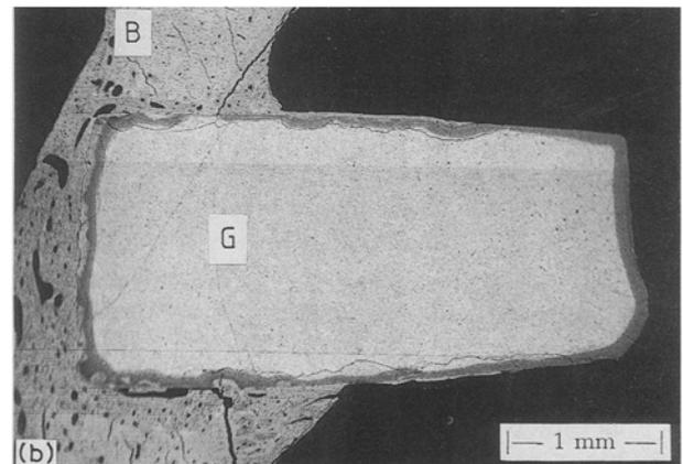
Figure 8 (a, b) SEM micrographs of the phosphate-free glass S46P0 showing bonding after 8 weeks in rabbit tibia. Phosphate from the surroundings has penetrated into the glass surface and a calcium phosphate surface has formed. The calcium phosphate-rich layer is non-uniform. G = bulk glass, Si = silica-rich layer, CP = calcium phosphate-rich layer, B = bone.
