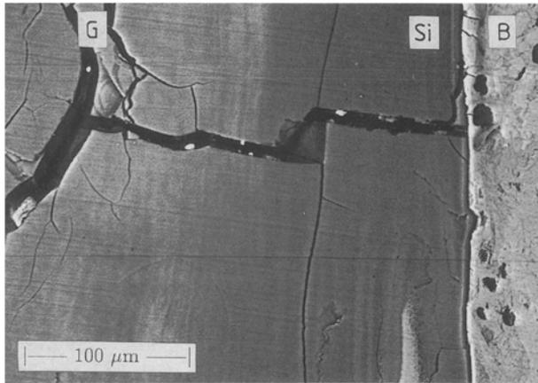
Figure 5 SEM micrograph of glass S52P8 showing contact, but no bonding, after 8 weeks in rabbit tibia. G = bulk glass, Si = silica-rich layer, CP = calcium phosphate-rich layer, B = bone.
