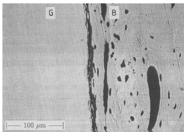
Figure 3 SEM micrograph of glass S65.5P1 showing poor or no contact after 8 weeks in rabbit tibia. G = bulk glass, B = bone.
