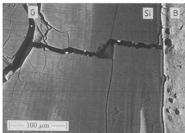
Figure 4 SEM micrograph of glass S52P3 showing contact, but no bonding, after 8 weeks in rabbit tibia, G = bulk glass, Si = silica-rich layer, B = bone.
