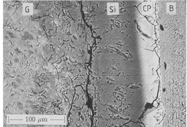
Figure 7 SEM micrograph of glass S55.5P4 showing bonding after 8 weeks in rabbit tibia. G = bulk glass, Si = silica-rich layer, CP = calcium phosphate-rich layer, B = bone.
