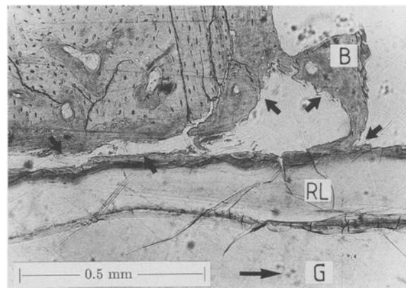
Figure 2 Optical micrograph of glass S46P0 after the push-out. Fracture occurs in the bone (B), whereas bone is still adhering to the glass (RL = reaction layer, G = bulk glass). Long arrow indicates direction of loading and short arrows the fracture line.
